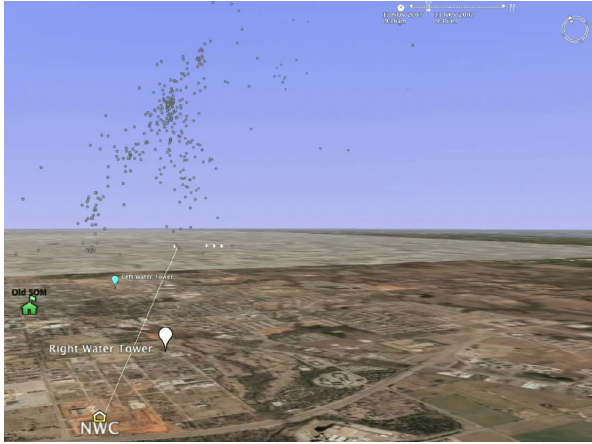
Figure 3a. VHF source locations at ~ 10.848 seconds, the time of the NLDN located first stroke.
