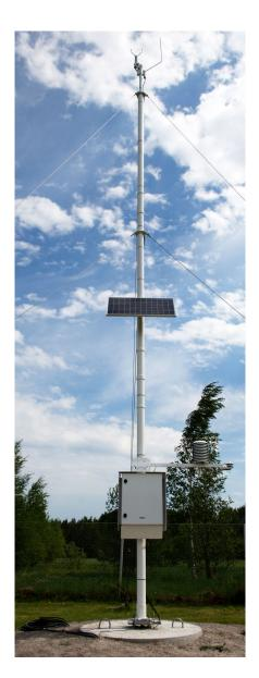
Vaisala Composite Pole Mast DKE110 is a 10-meter (33-feet) mast that is available with white (DKE110W) and with red/orange and white (DKE110AV) painting. The mast is suitable for a wide range of surface weather and climatological applications.
