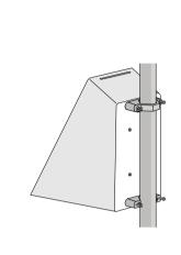
3.2 Attach PSU502 with solar panel frame to the pole mast.
