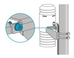
1.3 Attach AQT530 to the mounting bracket. Tighten the screw and nut to keep AQT530 firmly in place.
