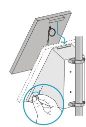
3.3 Tighten all bracket screws. Slide the solar panel to the holder and tighten the screws inside the holder
