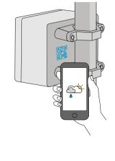
5.2 Scan the QR code on the back of the gateway to access read-only view of the measurement data in Wx Beacon.
