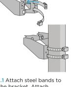
1.1 Attach steel bands to the bracket. Attach bracket to the pole mast and tighten the screws in steel bands.
