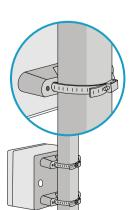
2.3 Tighten all screws evenly to keep power supply unit or gateway firmly in place.
