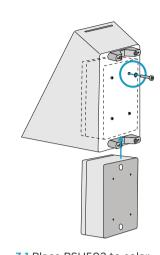
3.1 Place PSU502 to solar panel frame and secure with 4 screws. Attach 2 pole mount brackets to the frame with 4 screws.
