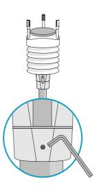
2.5 Tighten the fixing screw to keep the sensor firmly in place.
