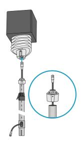
2.1 Place mounting kit to the top of vertical tripod mast.
