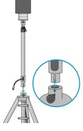
2.3 Attach the telescopic mast to the tripod. Tighten the screws with fingers.
