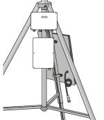
3.3 Slide the solar panel to the brackets. Tighten the screws.
