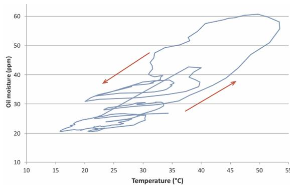
Figure 1. Online moisture monitoring data in ppm during temperature fluctuation in a 10 MVA (ONAN) transformer
