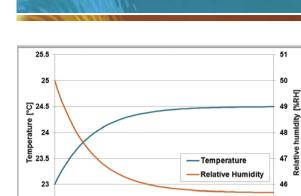
Figure 2: Example of a self-heating test. The transmitter is allowed to reach equilibrium with the surrounding environment.
