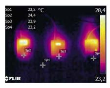
*Figure 4: Transmitter temperatures 30 minutes after power-up.*
