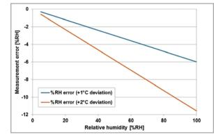
Figure 1: Error in relative humidity reading resulting from  $+1^{\circ}C$  (1.8°F) and  $+2^{\circ}C$ (3.6°F) self-heating at room temperature (20°C, 68°F).
