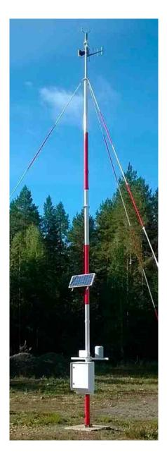
Vaisala Guyed Frangible Mast DKE110F is 10 meters (33 feet) high and suitable for a wide range of surface weather and climatological applications, including locations at the airports.
