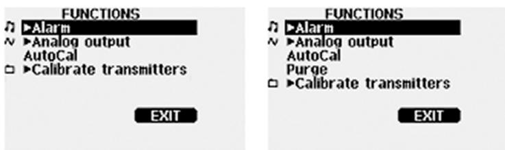
Figure 7 Functions menu for DMP74A (left) and DMP74B/C (right)
