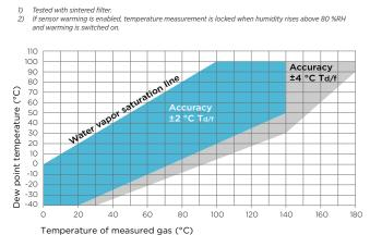
Dew point accuracy vs. measurement conditions
