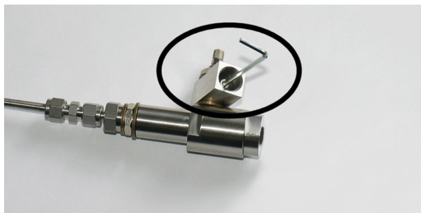
Figure 16 Removing the Leak Screw
