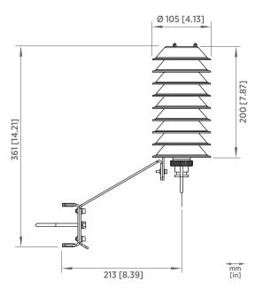
Solar Radiation Shield DTR502B dimensions
