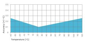
HMP9 temperature measurement accuracy over full
