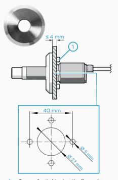
Screws for tightening the flange in place (4 pcs, Ø 5 mm)
