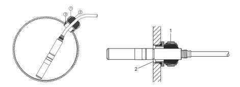
HMP247CG: Vapor-tight installation with cable gland.
