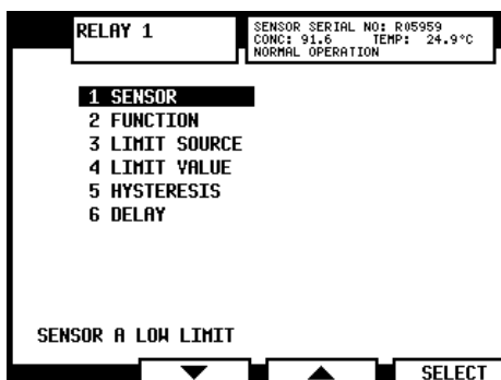
Figure 33 Relay menu for relay 1
