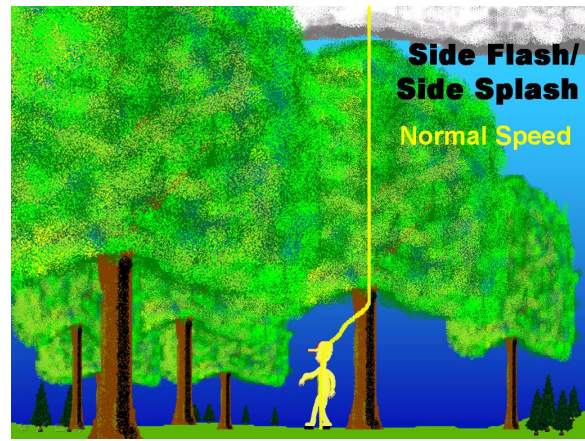
Figure 4. Example of a “side flash” from lightning striking a nearby tree.
