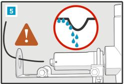
If wiring from above, note that moisture can move down along the cable to the connectors. Make sure moisture has no direct downward path to MMT162.
