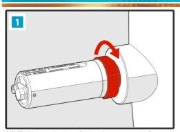
MMT162 must be installed to the process before attaching the weather shield. Tighten only from the 30 mm nut, never from the transmitter body. See MMT162 User's Guide for installation instructions.
