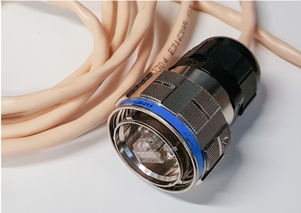
Figure 22 RJ45 connector inside the protection shell
