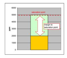
Gearcase Lubricating Oil Temperature: 70 °C Saturation point: 5000 ppm Actual amount of water in the oil: 2000 ppm a..: ~0.40
