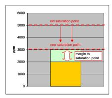
Gearcase Lubricating Oil Temperature: 30 °C Saturation point: 3000 ppm Actual amount of water in the oil: 2000 ppm a<sub>m</sub> ~0.67
