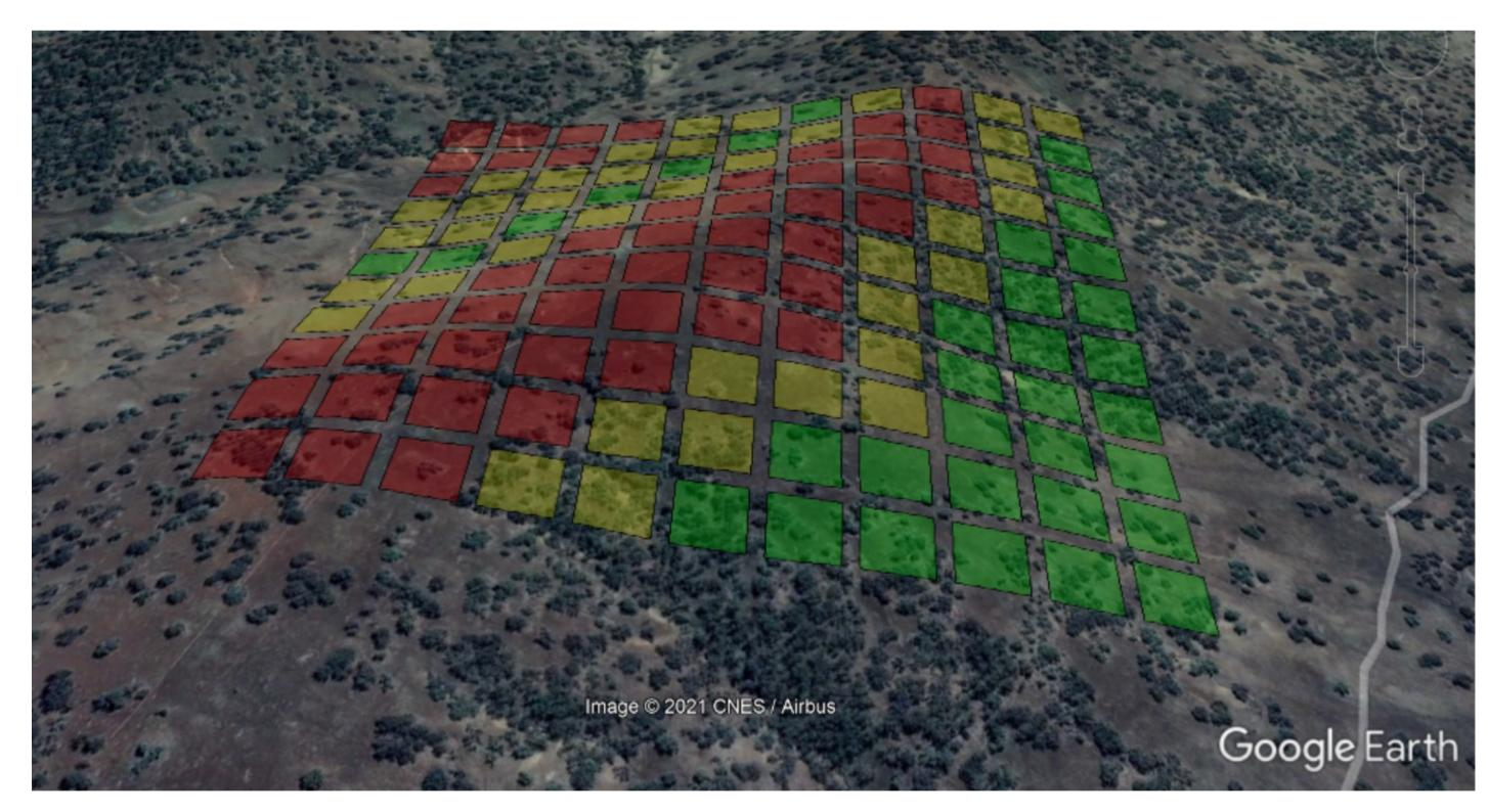
Green locations predict an error below 1% where no correction is suggested to the wind lidar measurements.
