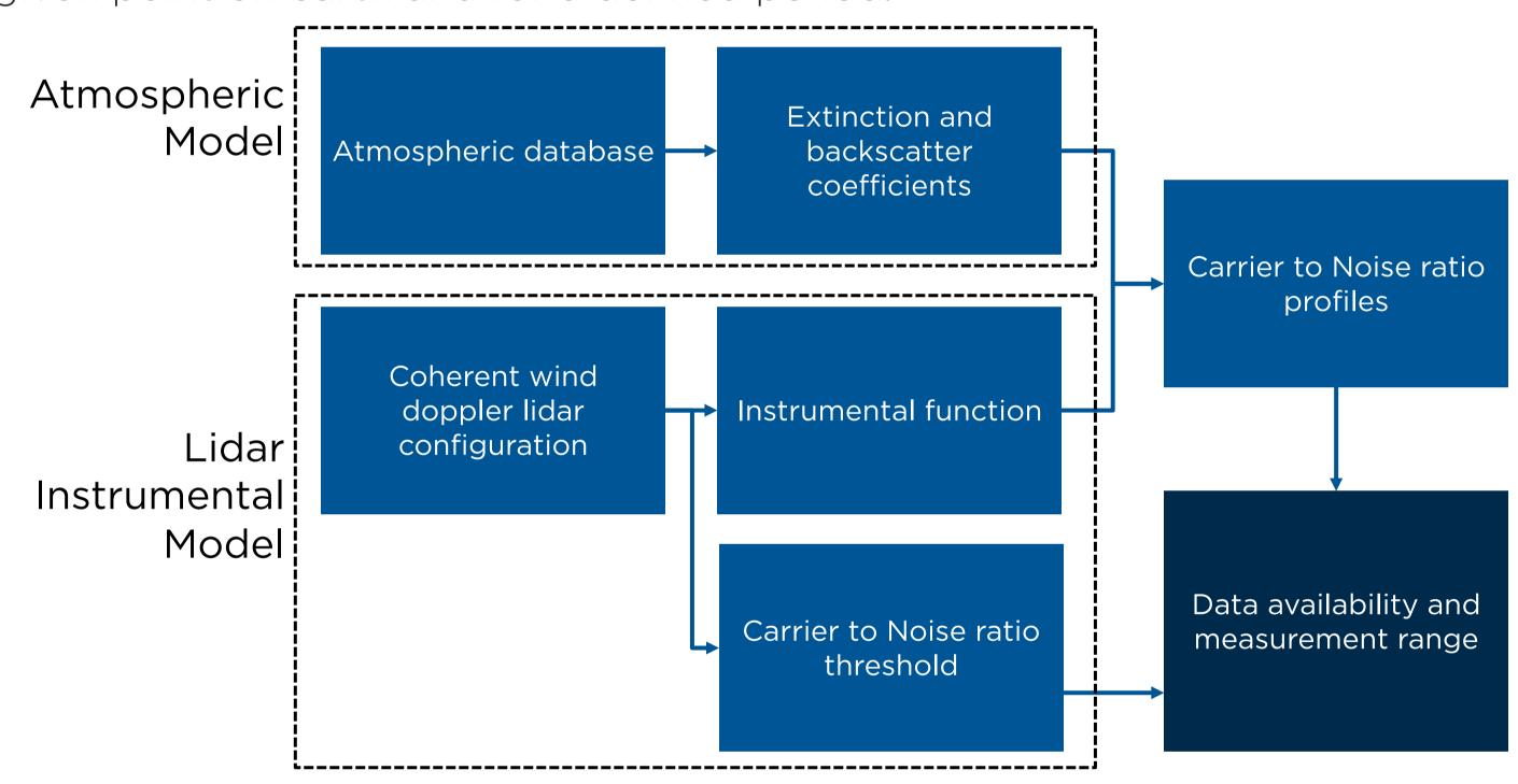
NB: Extinction and backscatter coefficients are computed using raw data from the ECMWF database and calculating the aerosol optical depth, boundary layer height, and lidar ratio parameters.
