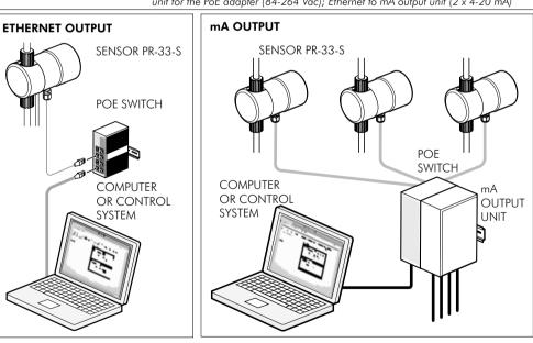
IEEE 802.3af compliant PoE switch (4+2 ports, 24Vdc/48Vdc input); Power supply unit for the PoE adapter (84-264 Vac); Ethernet to mA output unit (2 x 4-20 mA)
