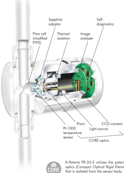
K-Patents PR-33-S utilizes the patented COREoptics (Compact Optical Rigid Element) module that is isolated from the sensor body. The integral probe type temperature sensor responds fast to the changes of the process liquid temperature. The CORE-optics protect the measuring components from any influence of pressure, flow or temperature changes.
