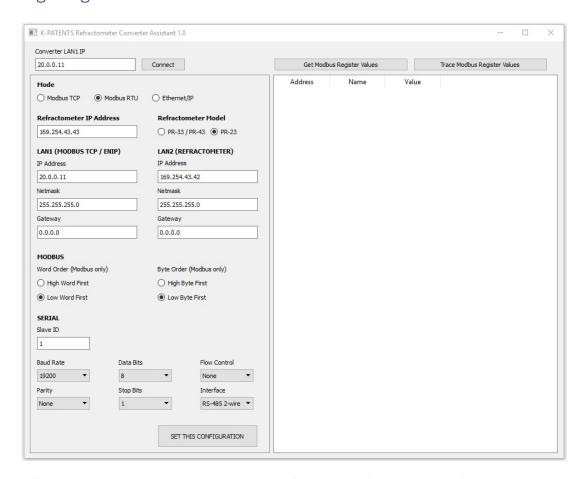
To configure the converter, use the provided software tool "K-PATENTS Refractometer Converter Assistant".
