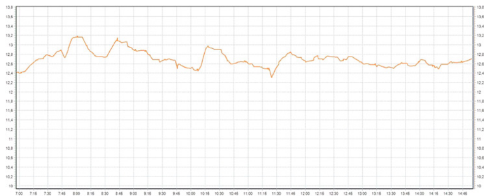
Figure 6 Example of a control chart showing TDS content in the pulp feed to a fiberline. This data is obtained only by K-Patents Process refractometers.
