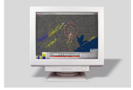
In the main application, lightning warning areas and electric field mills are monitored in real-time. Remote alarm displays, e-mail notifications, and relays are triggered once the TWX300 workstation issues a lightning warning.
