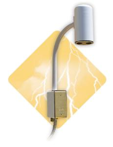
Up to 7 on-site Vaisala Electric Field Mills can be added to monitor overhead lightning potential. Vaisala Electric Field Mills measure the actual electrostatic charge in the local atmosphere to show when conditions are ideal for lightning to occur.
