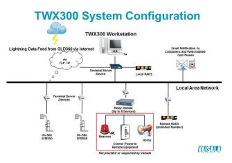
The typical Vaisala Thunderstorm Warning System TWX300 installation leverages an existing local area network to connect to the central lightning network and local electric field mill data sources. Alarms are distributed through the remote alarm displays (RADS), e-mail notification, and relays.
