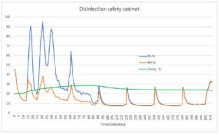
"The graphs show how important it is to know both the relative saturation and relative humidity during a process. This is especially true when disinfecting equipment that has HEPA filters.
