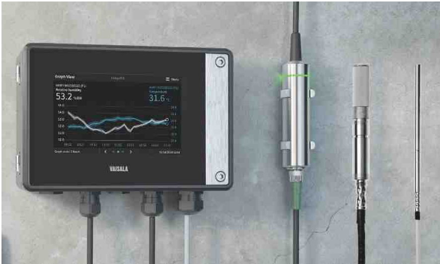
Indigo 520 transmitter with HMP7 humidity probe body and sensor head and TMP1 temperature probe in the far right.
