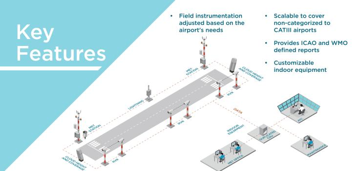
A typical AWOS solution consists of the field sensors, central data unit(s), communication interfaces and different workstation types.
