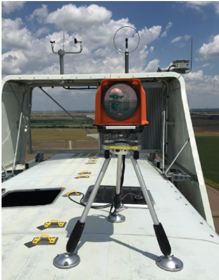
Installation of Wind Iris 4-beam (earlier version of WindCube Nacelle)
