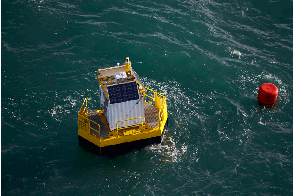
Figure 11: WindCube Offshore deployed on a buoy – The sunshade helps protect the lidar window against solar radiation, dejection, and splash in offshore deployments. Photo courtesy of Akrocean.
