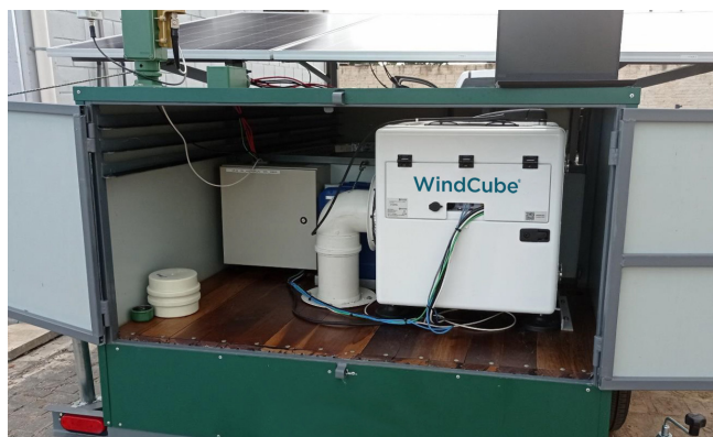
Figure 17: WindCube integrated in a trailer with a cooling system attached to the lidar – Photo courtesy of Hobeco.
