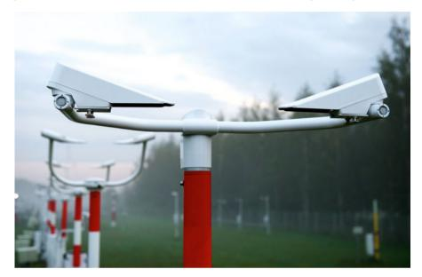
The Vaisala Forward Scatter Sensor FD70 is a powerful technology that can outperform and potentially replace the functionality of many separate sensors, such as a present weather sensor, rain gauge, disdrometer, and freezing rain sensor. The FD70 helps you make the best decisions for safer runway operations, even in the most challenging weather conditions.
