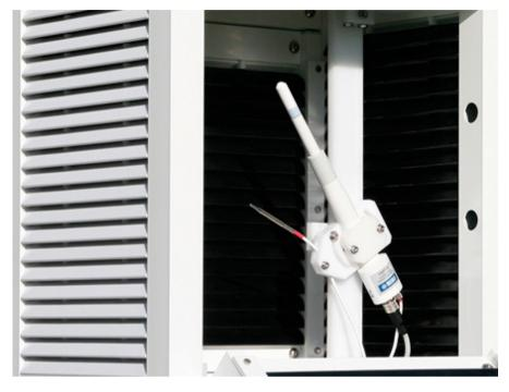
In high humidity climates where moisture is near saturation and in environments with changing temperatures, capturing accurate data is especially challenging. These are the types of conditions for which Vaisala's HUMICAP<sup>\*</sup> Humidity and Temperature Probe HMP155 were specifically designed.
