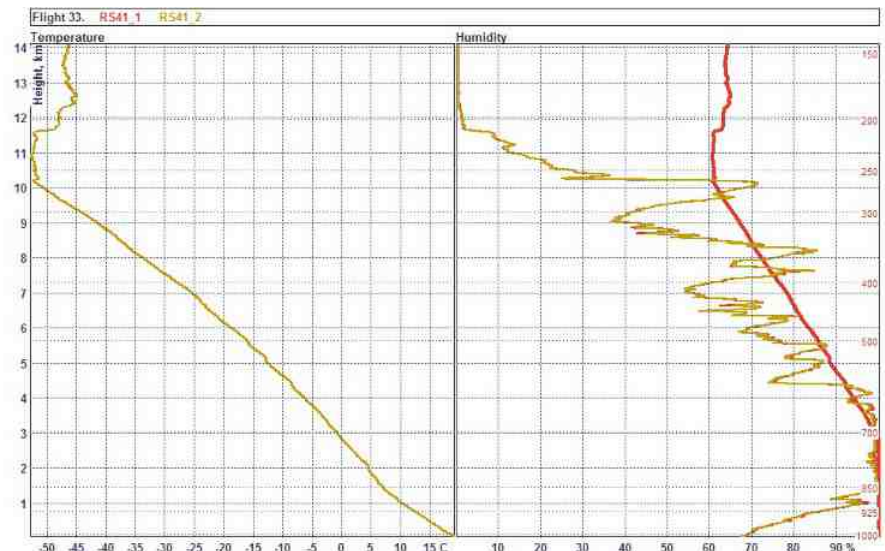
Figure 3.4. An example of a challenging sounding profile for humidity measurement at high latitudes during daytime. The thick red profile indicates a saturated RH level. The RS41 units (thin red and beige profiles) show good measurement consistency.
