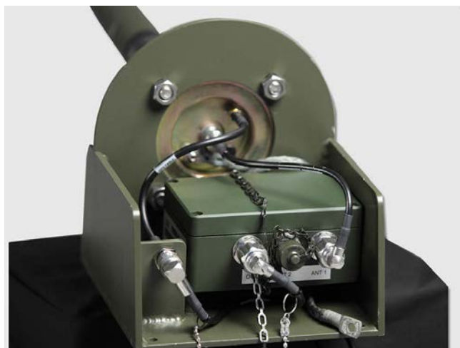
CG32 internal and external cables
