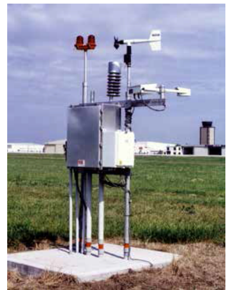
RWIS installed on an airfield - weather station with sensor suite (atmospherics)
