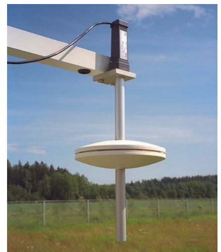
PTB210 paired with SPH10 static pressure head
