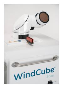
Vaisala WindCube Scan performs 24/7 real-time wind and aerosol measurements and high-level data processing using Doppler pulsed lidar, providing comprehensive information on airborne dust levels, their travel and their exposure to nearby communities for an effective means of operational excellency through better air quality.
