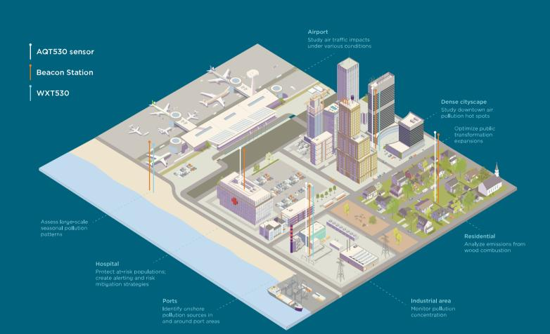
In this sample network, AQ and weather sensors work in harmony and can be placed freely — and cost-effectively — for highly localized insights. They can integrate with existing network infrastructures or utilize Vaisala's cloud-based system, depending on user needs.
