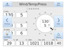
WID513 weather panel display closeup of a clear, uncluttered user interface for simple operation
