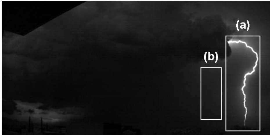
Figure 1. Example of (a) flash and (b) calibration areas of a high-speed video frame that recorded a long CC (considered in this study).
